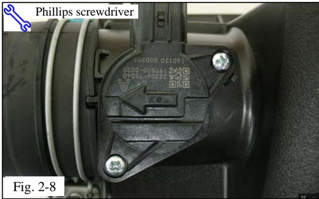
(h) On a workbench, remove the MAF sensor from the OEM air box by removing the two screws (Fig. 2-8).
