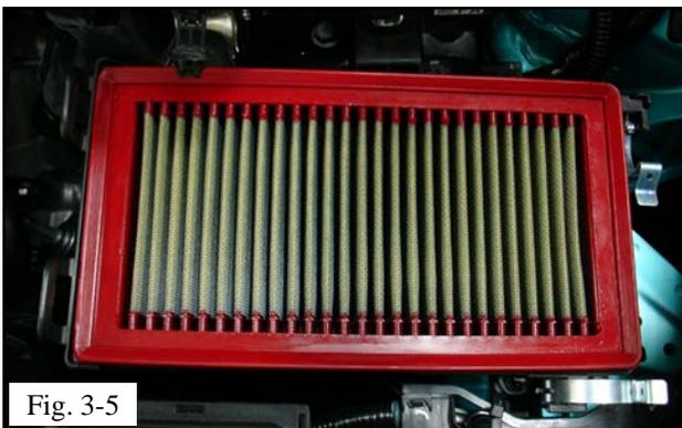
(e) Install the TRD air filter. Noting proper orientation by matching the square corner of the air filter to the proper corner of the OEM lower air box (Fig 3-5).
