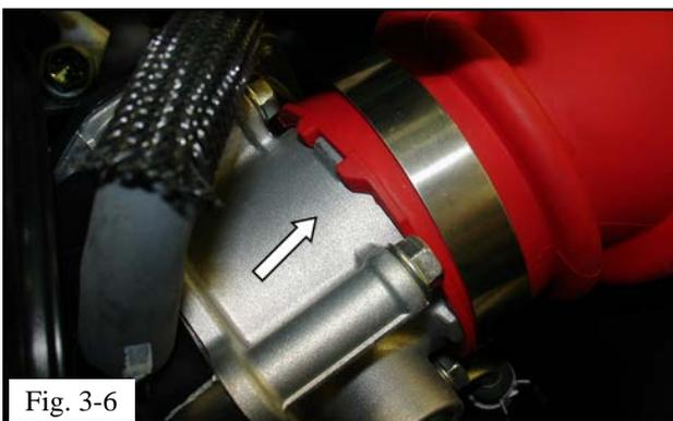
(f) Install the TRD coupler loosely on the throttle body (Fig 3-6).
