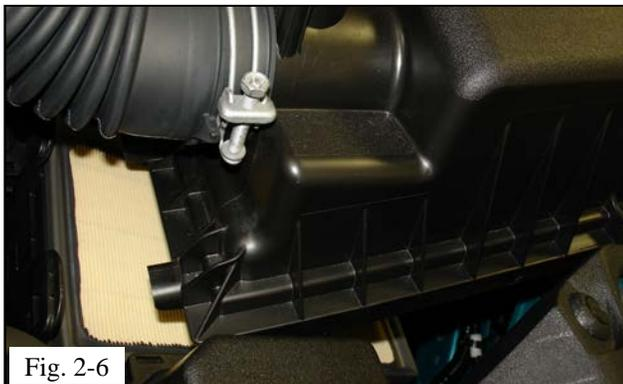
(f) Lift and remove the upper air box and coupler as an assembly (Fig. 2-6).
